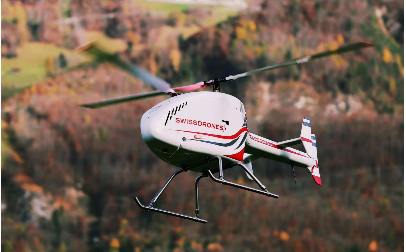
With a payload of up to 33 kilograms, SwissDrones' SDO-50 makes use of Flettner's intermeshing double rotors. Image: SwissDrones
