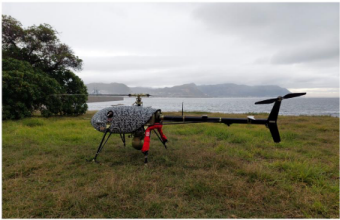
Figure 2. UVH 170 delivers georeferenced insights with dual visible-light and thermal cameras.
