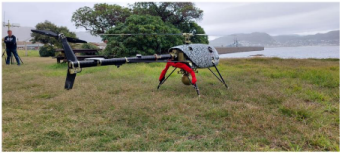
Figure 3. UVH-170 conducts aerial imaging and multi-level magnetic surveys, delivering geodata for pipeline construction.
