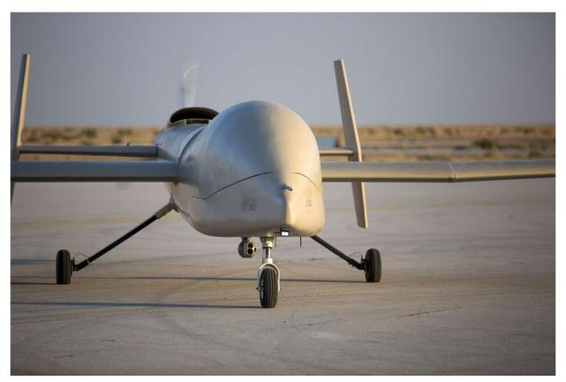
UAVOS and King Abdulaziz City for Science and Technology (KACST) in Saudi Arabia have developed the Saker-1B MALE UAV. It can fly for more than 19 hours at an altitude of up to 16,500 ft with a range of 2,600 km. (UAVOS)
