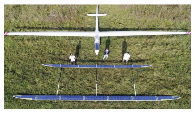
UAVOS successfully flight tested a 14 m wingspan version of its ApusDuo solar powered high altitude platform system (HAPS), pictured below. (UAVOS)
