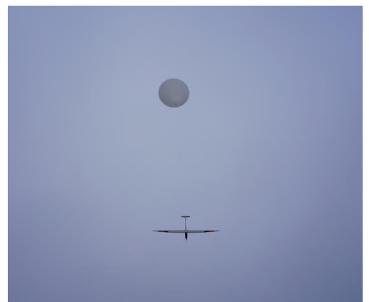
The HiDRON unmanned research glider is lifted aloft by balloon for release in the stratosphere. Credit: UAVOS
