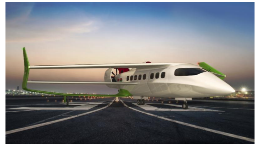
UK startup Faradair is designing the 18-seat biofuel hybrid-electric BEHA M1H for regional and cargo flights. Credit: Faradair
